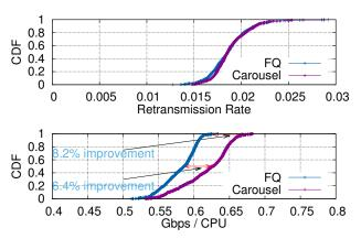
Figure 21: Comparison between FQ and Carousel for two machines serving large volumes of video traffic exhibiting similar CPU loads showing that Carousel can push more traffic for the same CPU utilization.
