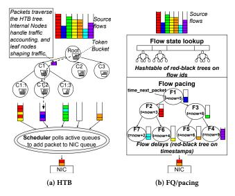
Figure 2: Architecture of Linux rate limiters.
